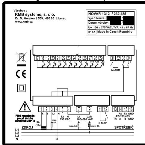
Fig. 2 : Three-phase capacitor wiring
