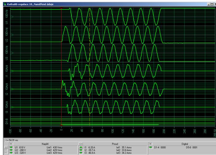
Figure 6: example of three-bank compensation, one KATKA 20T 25 kVAr + two KATKAs 80T, 45 kVAr
