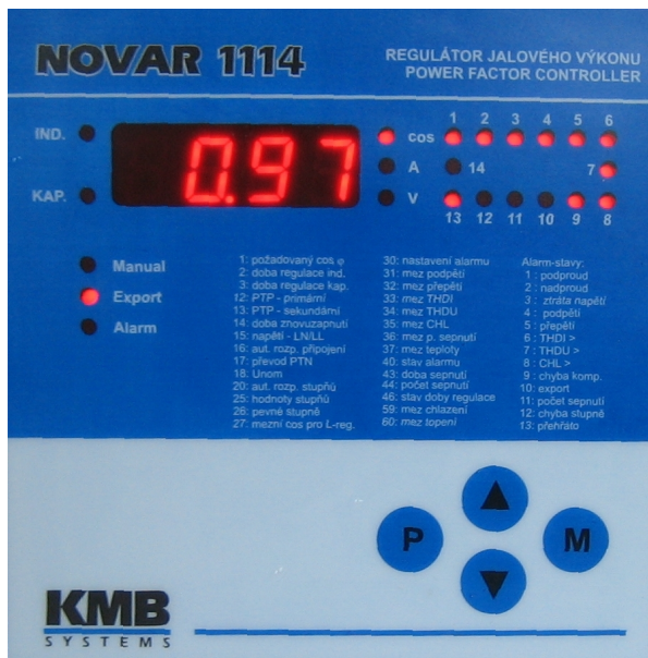
Fig. 4: Front side of the APFC NOVAR 1114, up 14 steps, keyboard configurable parameters
